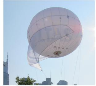
Figure 1. Kingfisher aerostat. The model being used for these measurements is 8 feet in diameter and 7 feet tall with a 1.5 to 2kg payload capacity.
